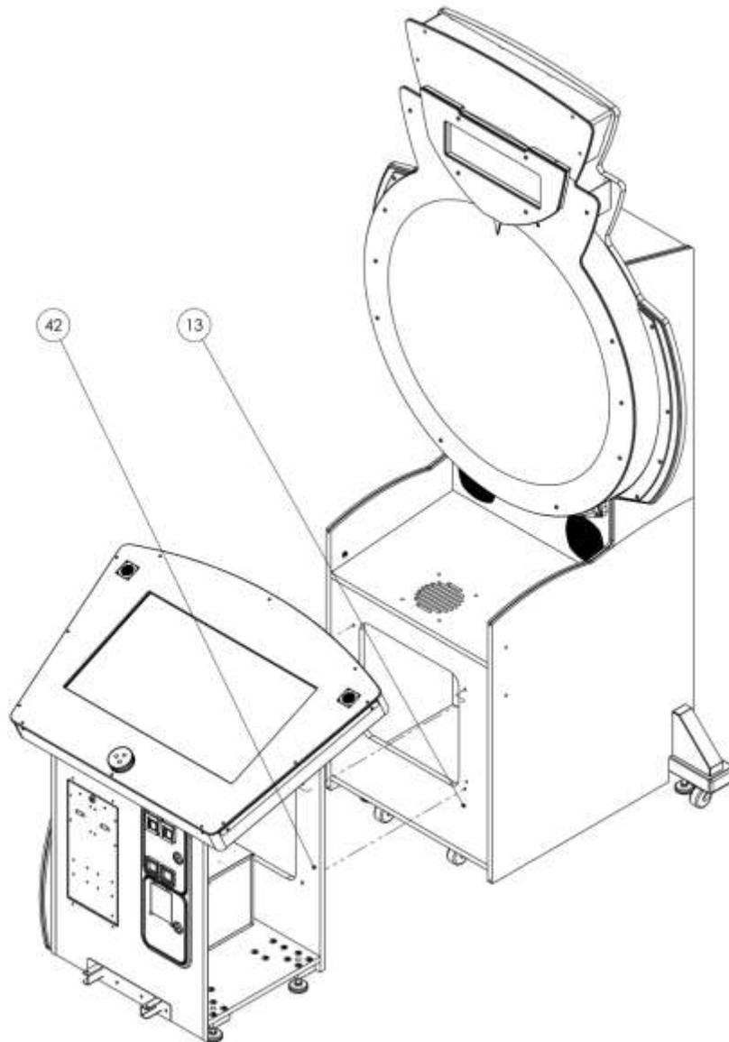
1. Push the monitor console toward the main cabinet and align the holes together.
