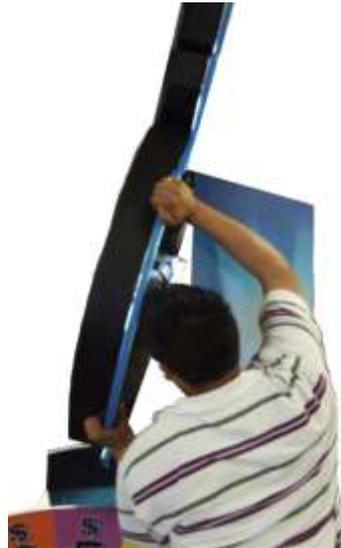
2. Slowly allow wheel to pivot into position. *Use extreme caution while wheel pivots. Be certain wheel is correctly positioned before releasing.*
