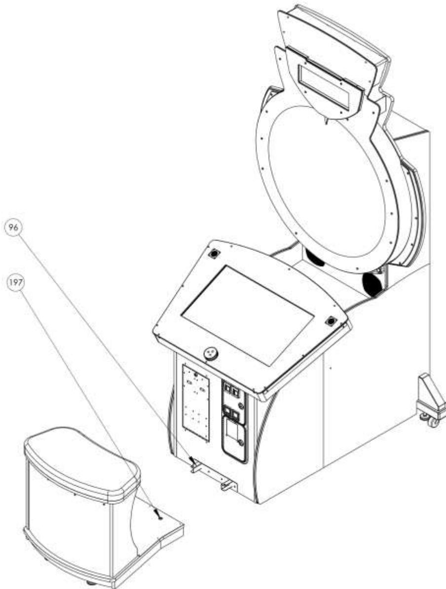
1. At the base of the display console front, locate the connector bracket (96).
