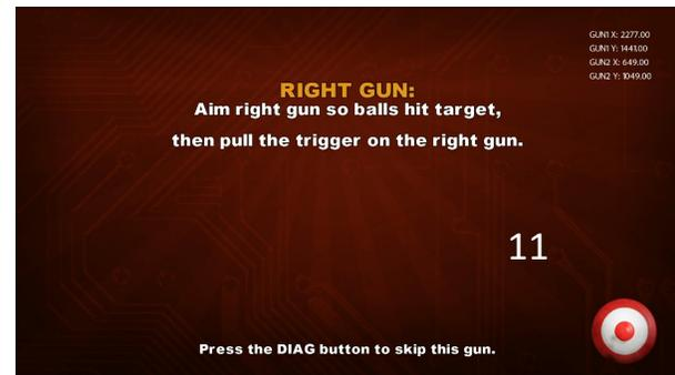
Now test the right shooter to ensure that the balls land near the rectangle in all areas of the screen [12]. If not satisfied, restart the test by pressing the “TEST” button.
