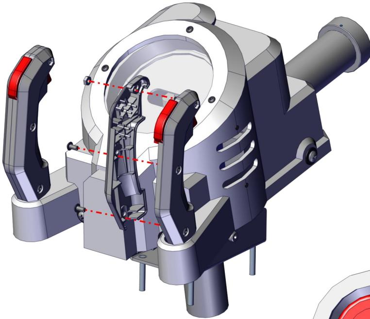
The handle is sold complete. Its part number is GB2006. When replacing, do not remove the rubber band holding the two halves together. Slide the new handle on top and remount.
