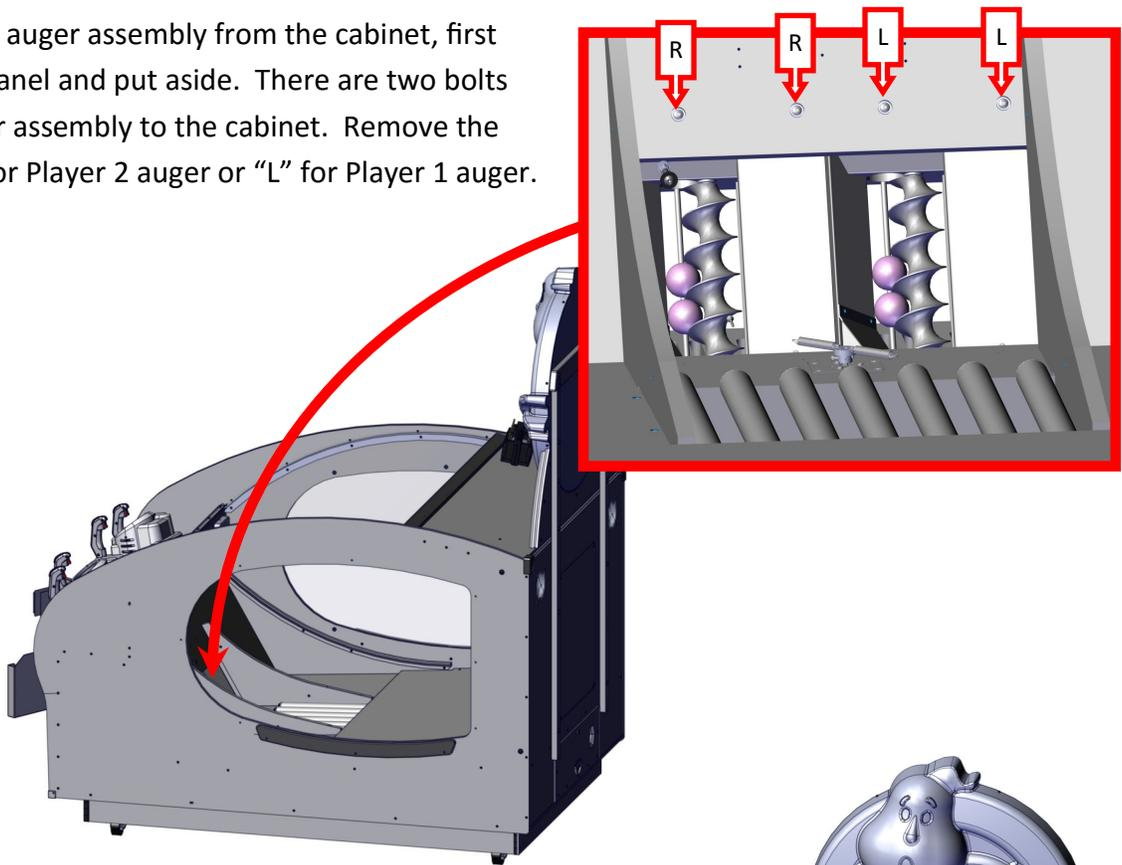
Open the front of the cabinet and loosen the 1/4 " hose clamp that holds the tube to the auger you wish to remove. Lift the tube up and out of the way. The auger assemblies sit in a slot at the bottom of the cabinet. Lift the auger up and unplug the two pin connector. Now remove the auger.
