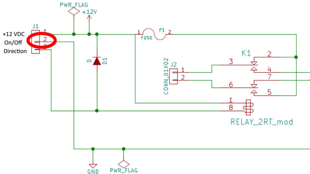
The ball auger direction is controlled by pin 20 of P7 of the I/O board for Player 1 and pin 21 of P7 of the I/O board for Player 2. This signal connects to pin 3 of the relay board. When this signal is low, it will activate the relay therefore reversing the power to the auger.
