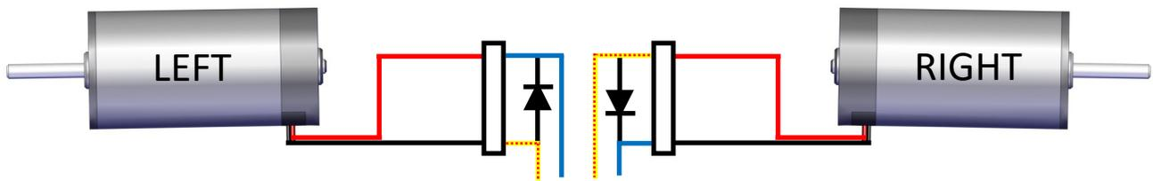
If +12 VDC is present at the motor but the motor is not running then a motor failure has occurred. To remove the motor, refer to the previous page for procedure.
