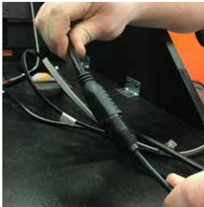
Plug in the 1714 cable housing into the 4003 cable housing.
