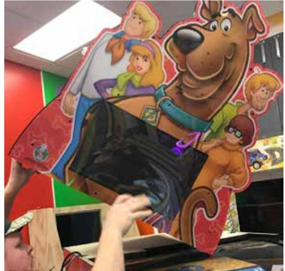
On the left side of the cabinet, lift the sleigh/marquee up and route the VGA cable and the 1709/1714 cable bundle through the cut out on the bottom of the sleigh/marquee.
