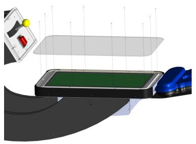
Remove the back cover and disconnect the DC power from the +24 volt power supply and the DVI video cable to the monitor.
