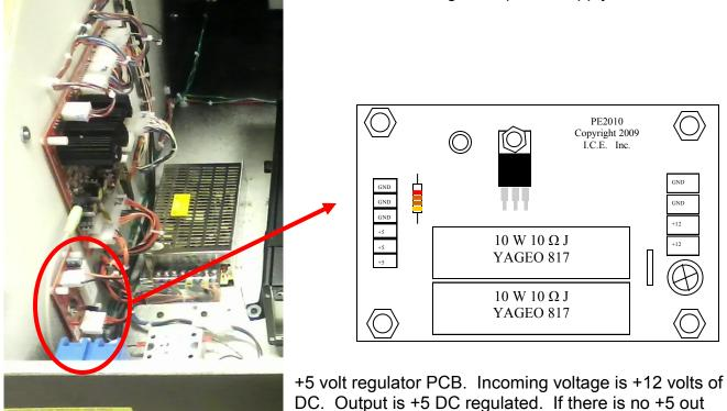
DC. Output is +5 DC regulated. If there is no +5 out check for +12 DC in or +12 out from PE2010X. If +12 is also missing, check 110v in to PE2010X power supply.
