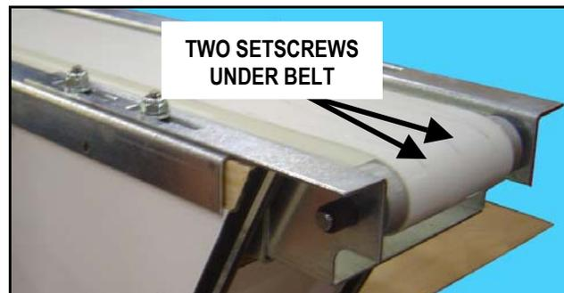
Figure 10 Belt Removal – Exit End
