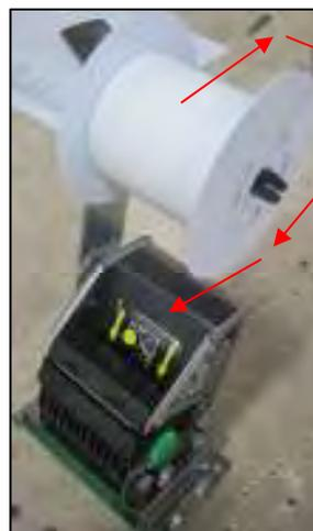
Note: Paper must feed under holder and into printer
