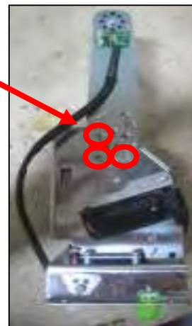
Place a side piece onto the core holder.
